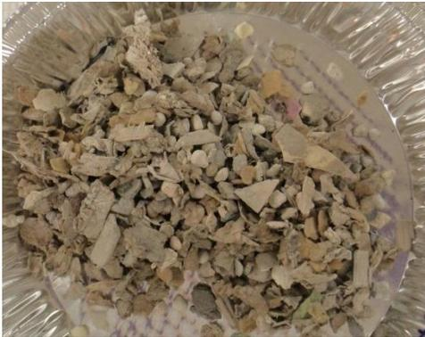
A photograph showing a large quantity of light-colored, irregular fragments of ceramic and porcelain in a silver foil tray. The fragments are larger than those in the previous images, with many pieces being angular and sharp-edged.                                   |
