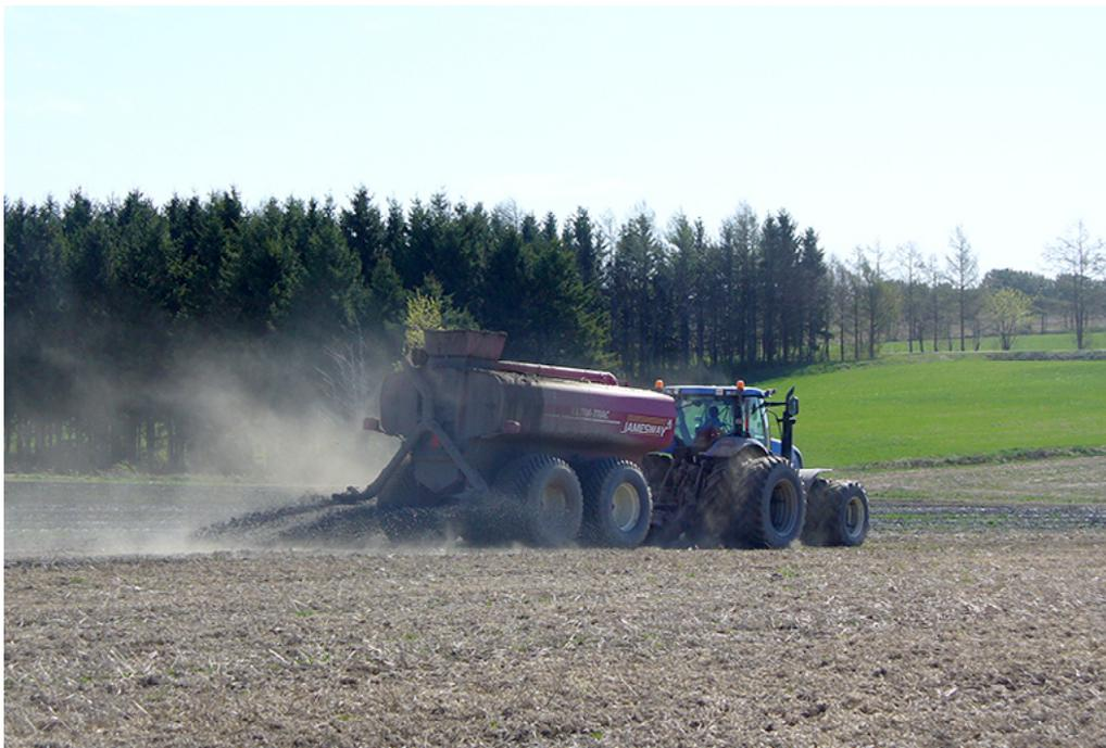
**FIGURE 4.3 : ÉPANDAGE DE BIOSOLIDES MUNICIPAUX AU PRINTEMPS AVANT LES SEMIS**
