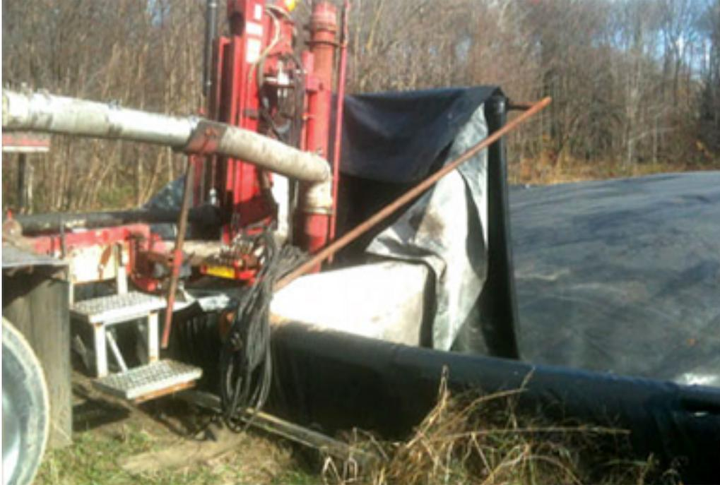
**FIGURE 3.10 : ENTREPOSAGE DE MRF LIQUIDES AVEC MATELAS FLOTTANT DE PAILLE**
