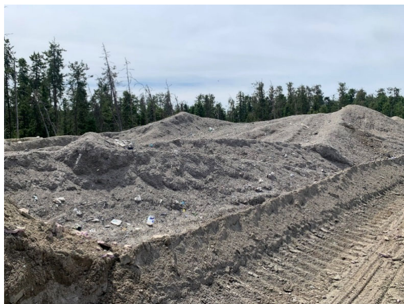
Figure 9: Granular materials generated during street cleaning work
