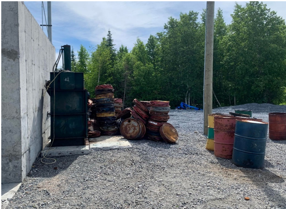
Figure 25: Hydraulic press for compacting barrels at the ecocentre in the Cree village of Mistissini
